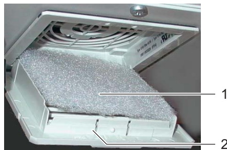
figure 5-16 Exchanging the lower filter mat
