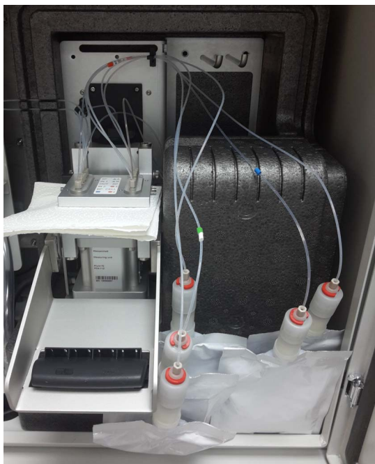
figure 5-20 Absorbent paper in the receptacle of the MultiPort valve
