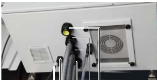
figure 3-24 Connections at the housing bottom (from below) Example: 2 sample channels, 1 drain
