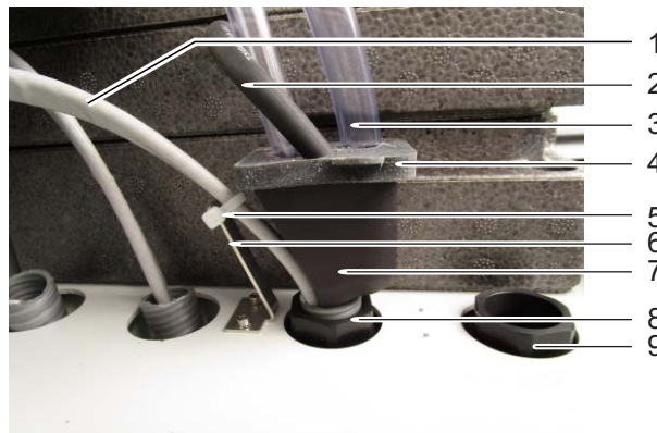
figure 3-25 Collection funnel for the common discharging of all liquids
